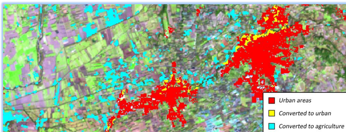
Figure 33. Distribution of classification errors in Dep. 84. False urban changes are located inside or close to exiting urban areas, while agriculture errors are scattered along the territory (from a visual point of view, this makes difficult the interpretation of the results).
