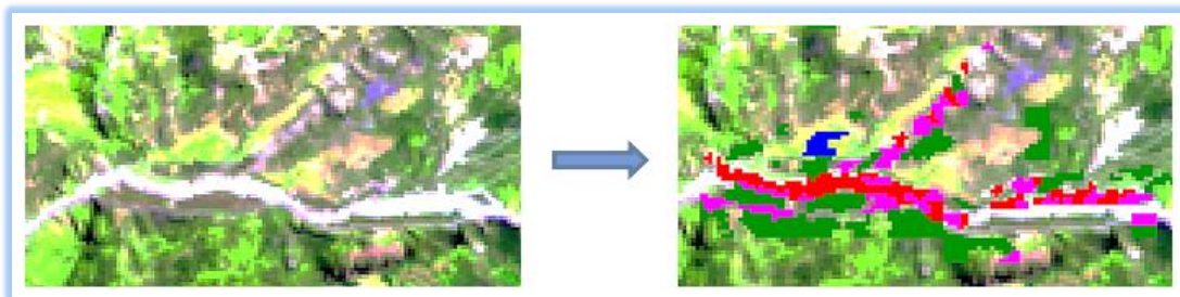
Figure 11. Supervised classification process for a Landsat 7 ETM+ image of the Dep.05 (August, 2001). It is possible to appreciate confusions between some classes. For example, the riverbed (red) and bare rocks (pink). The software also overestimates riparian forest class (green) or does not detect all the crops in the image (blue).
